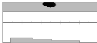
The same thick rusted iron bolt checked from a different direction, more clearly showing it is ferrous.
